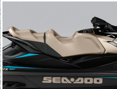
ERGOLOCK™ SEAT WITH STEPPED DESIGN
